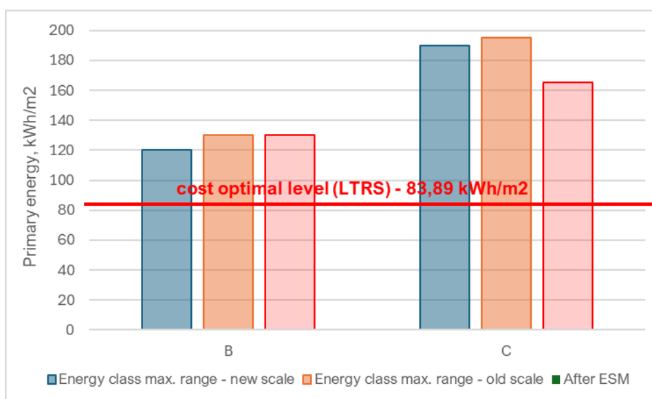
Figure 3. Average recommended renovation level for childcare facilities versus cost-effective renovation benchmark in LTRS
